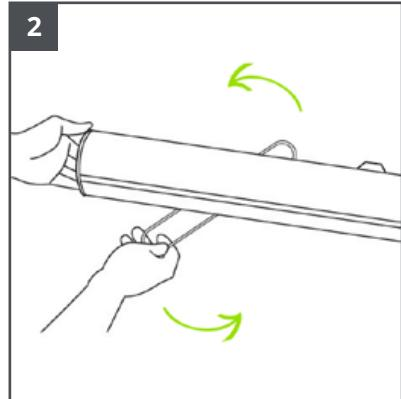
Pull the stabilizing feet out to be perpendicular with the base.
