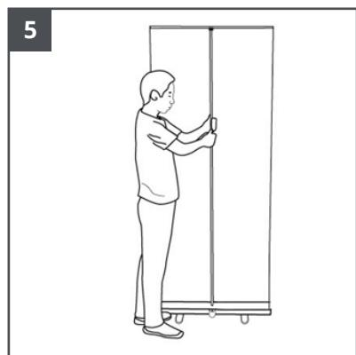
Adjust the height of the telescopic pole according to the length of the graphic.
