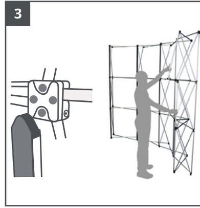
Install the magnetic channel bars into the vertical columns across the entire front of the display as well as the two rear edges of the frame.
