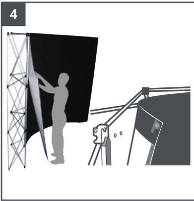
Hang panels by aligning magnets on top corners of panels to magnets on top hubs. Align magnetic tape on rear of panels to the magnetic channel bars.
