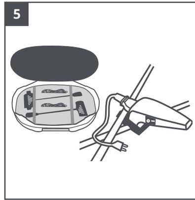
Install lights located inside the case lid by inserting the base of the light adapter into the 'X' created by the top horizontal cross bars of the frame.
