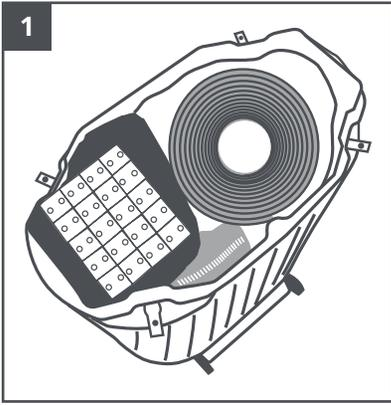
Open the transport case and remove the pop-up display frame and magnetic channel bars.
