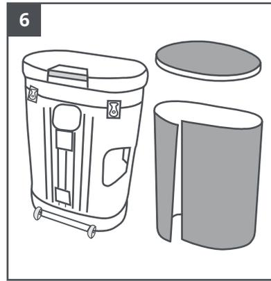
Convert your case to a podium by wrapping the podium wrap panel around the outside of the case. Place the hardwood oval on top of the case.
