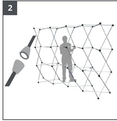
Ensure that the grey adjustable feet located on the bottom of the frame are facing the ground and pull the frame open until the magnetic locking connectors engage.
