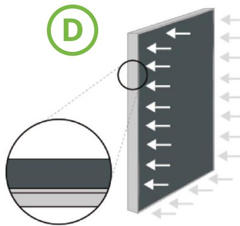
Work outwards towards the corners while continuing to press downwards on the silicone edging. To avoid stretching, creasing at the edges and dirtying the graphic, do not wipe your hands across the image.
