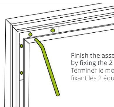
Finish the assembly of the frame on one side by fixing the 2 brackets.
