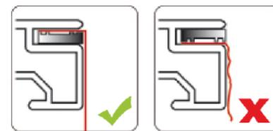
Insert the graphic in the 4 corners of the frame by pushing the silicone edging into the groove.
