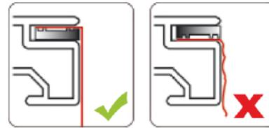
Insert the graphic in the 4 corners of the frame by pushing the silicone edging into the groove. Commencez par les 4 angles.
