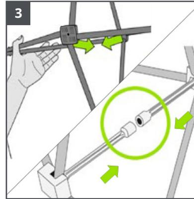
Pull the structure together at the cross-bars. The magnetic connectors will lock the frame into place.
